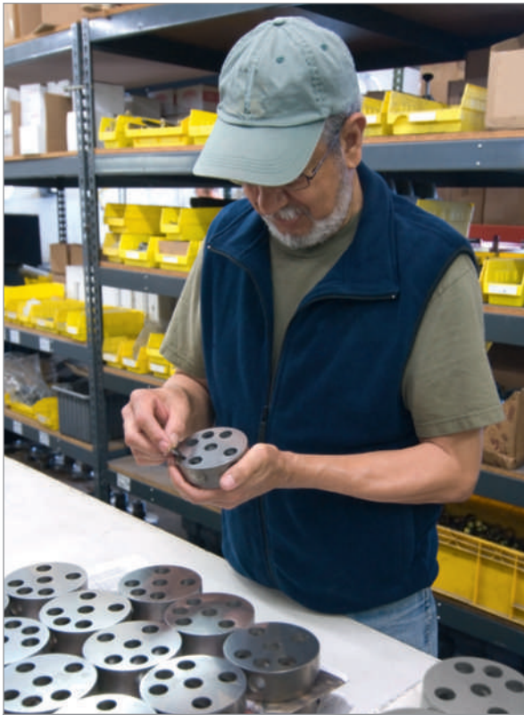
Process measurement is the key to quality improvement. Here a quality inspector measures the diameter of holes in a machined part.
