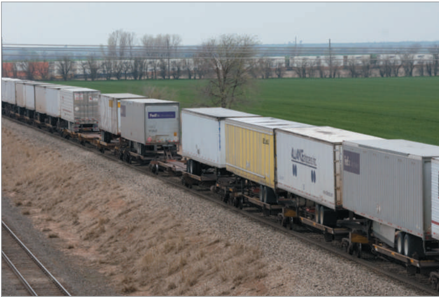
Truck trailers, often referred to as “piggy back” trailers, catch a ride on a BNSF intermodal freight train near Wellington, KS for a cross-country journey.
